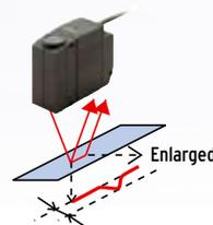
For detection of small recesses and protrusions in measurement location.
