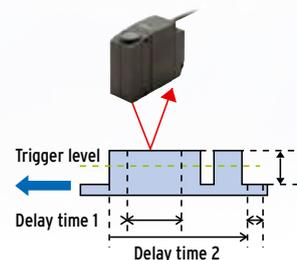
For measurement of steps in different locations with moving sensor or workpiece.
